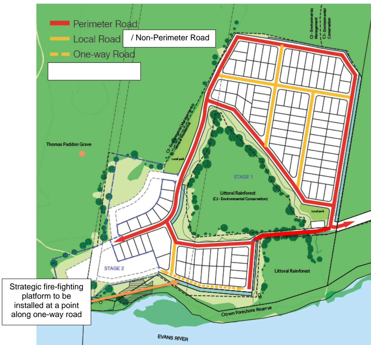
Figure 03: Street and Block Layout prepared by Dickson Rothschild and modified by the experts to nominate relevant classification of roads under PfBP
