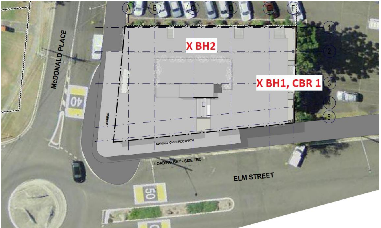
Plan of the site, with ASCT test positions.
