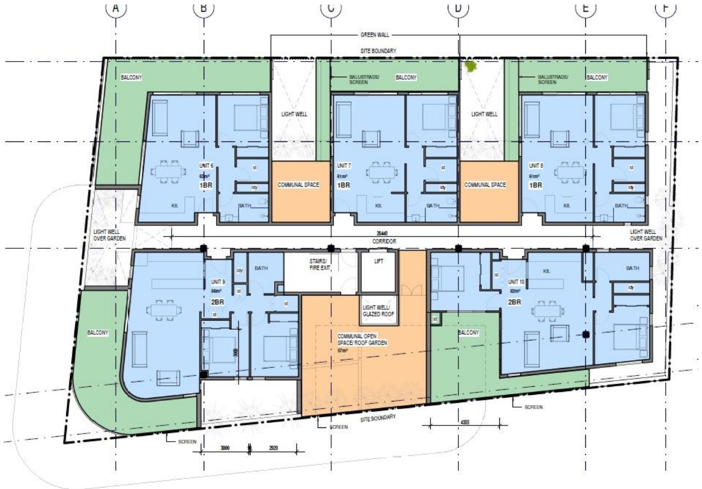
Figure 6 | Proposed layout, Second floor, Source: Barker Architects.
