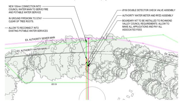
The fire hydrant system includes a new connection into the council water main, a double detector check valve (DDCV) and an external feed fire hydrant located a min. 10m away from the new building.
