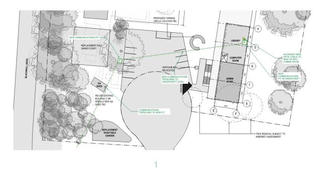
**Power:** Proposed power supply will be an underground cable from existing pole 3750 in the western boundary of the site next to the existing fence:
