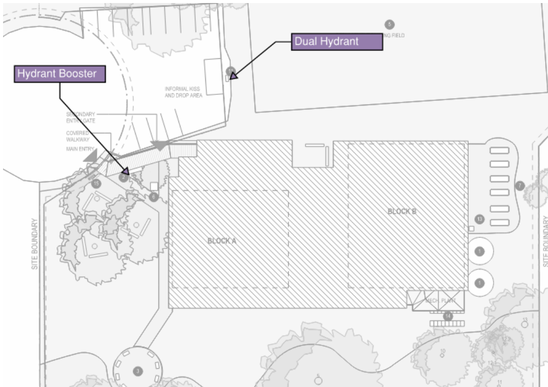
Figure 2: Location of the Dual Hydrant and Hydrant booster.
