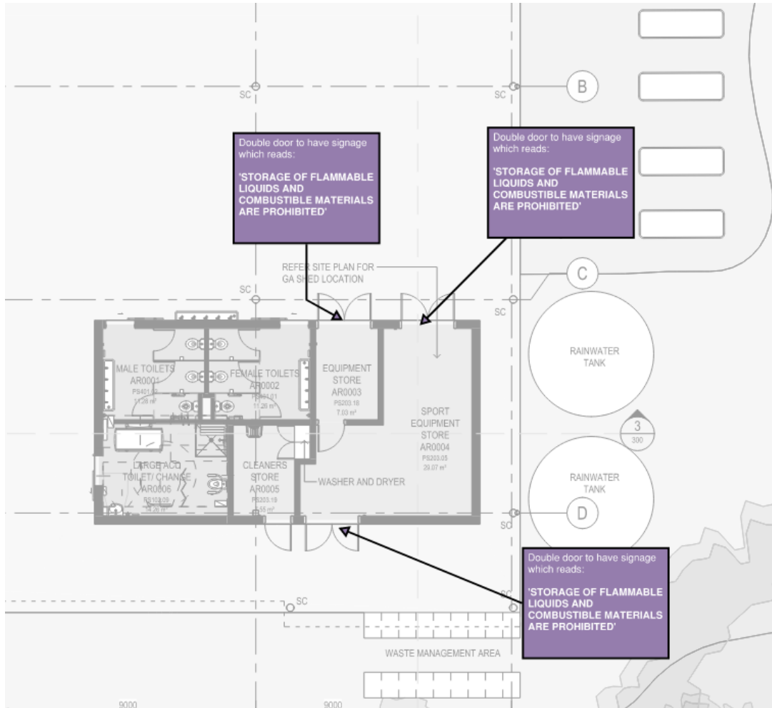
Figure 5: Indicative signage to double doors prohibiting the storage of flammable liquids or combustible goods in the undercroft storerooms.
