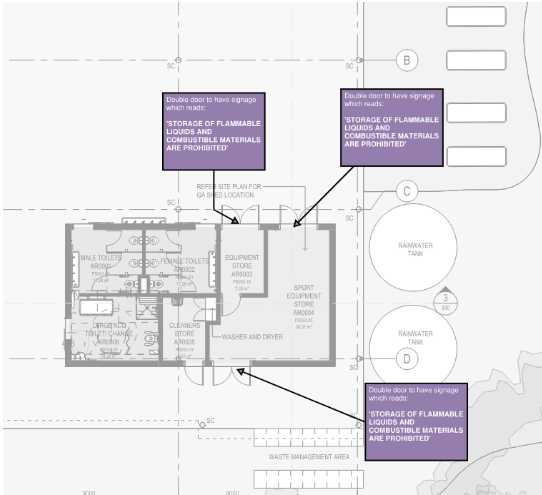
Figure 13: Indicative signage to double doors prohibiting the storage of flammable liquids or combustible goods in the undercroft storerooms.
