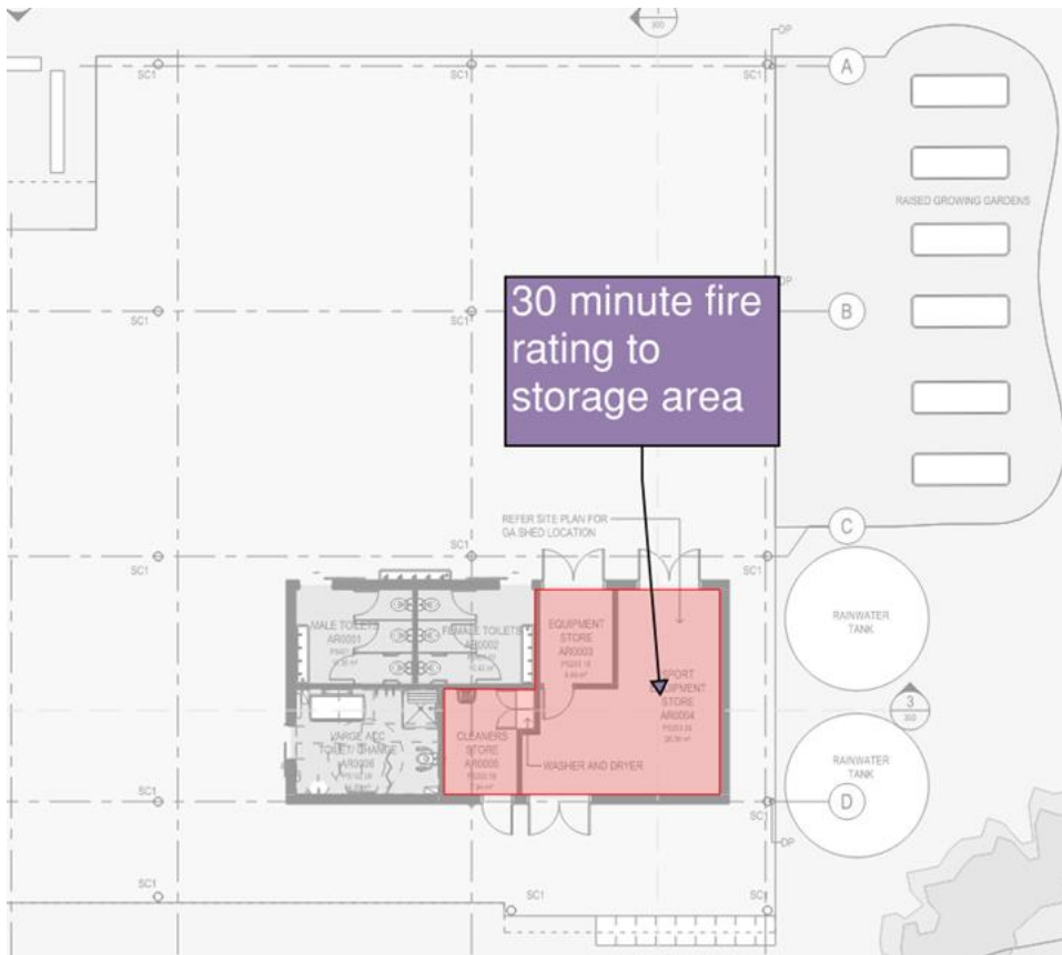
Figure 6: Storage area fire rating requirement
