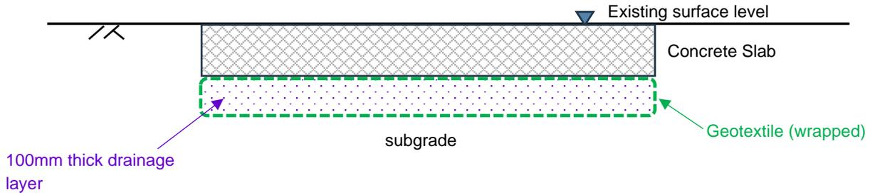
Figure 2: Sketch for proposed drainage layer under pavement
