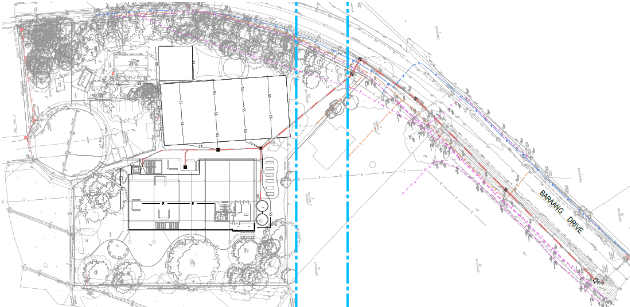
Figure 35: Proposed stormwater pipe system (Source: Henry & Hymas)
