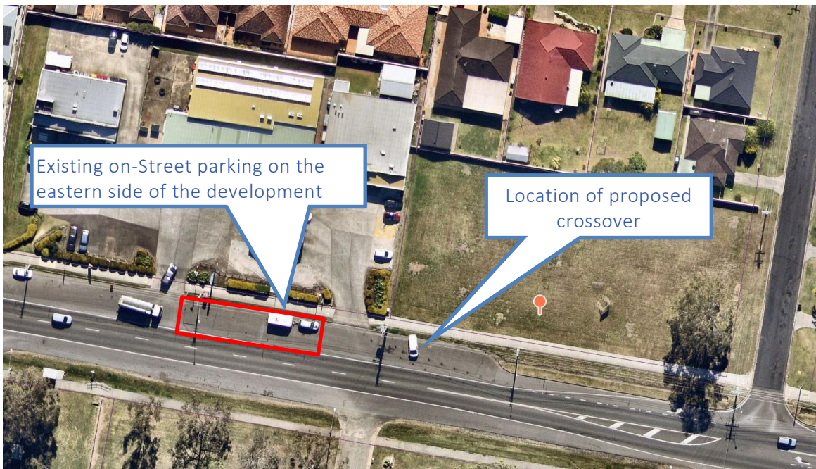
Figure 6.2: Existing on-street parking facility effect on the sight line
