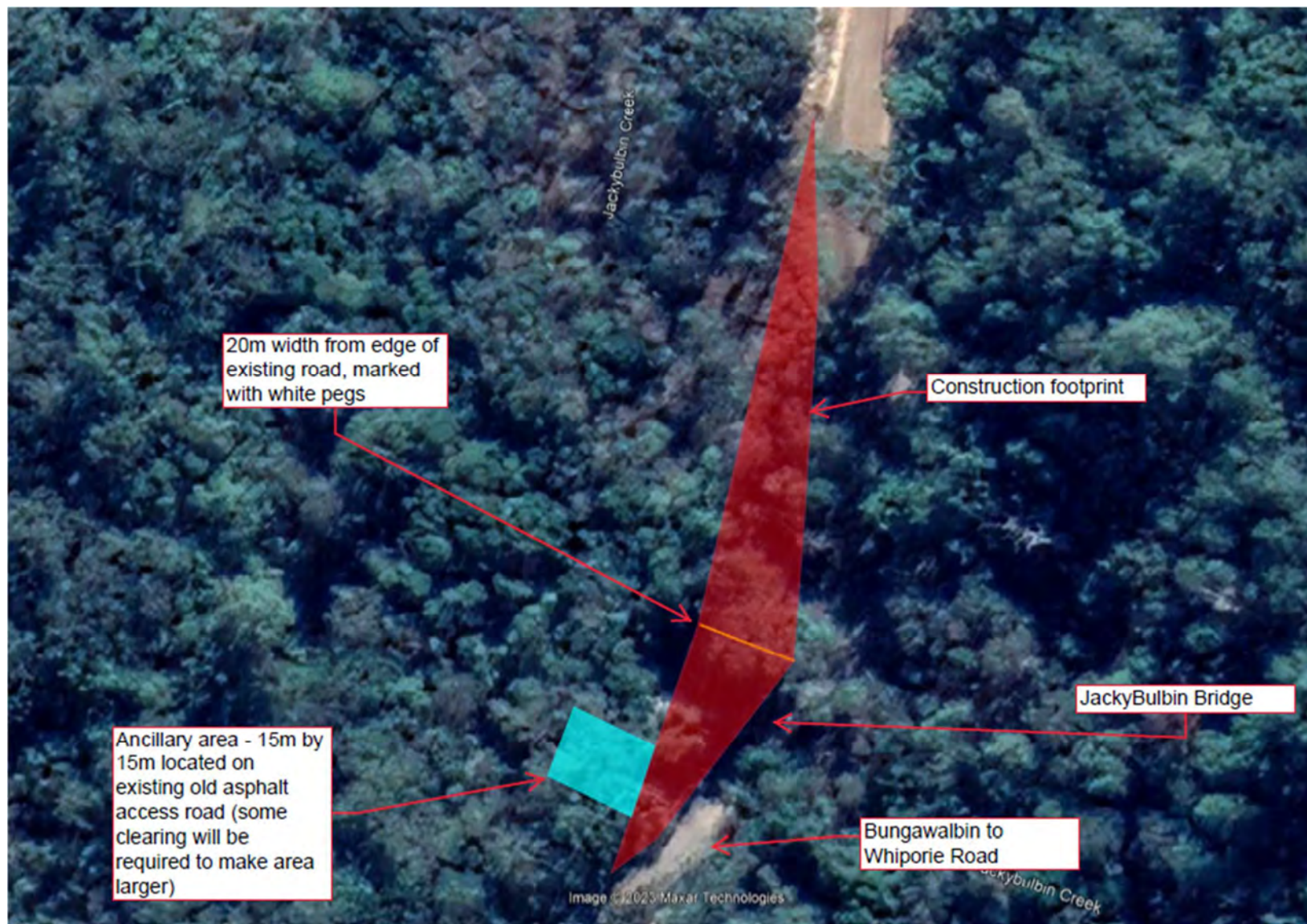
Figure 2: Location of Jackybulbin Bridge replacement in relation to the existing bridge (Envirocivil Consultants)
