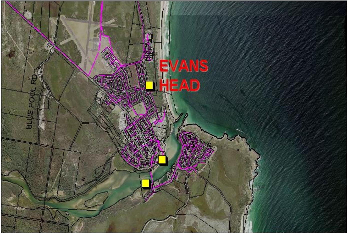
Reticulation constructed overflows
