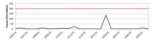
Figure 2.11 Time series of faecal coliform concentrations from the Evans Head STP discharge (90th percentile limit in red)
