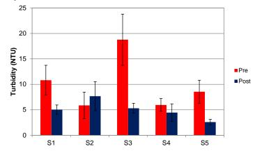
Figure 2.17 Mean ± SE turbidity measurements in discrete samples from surface waters at all sites before and after channel closure
