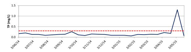
Figure 2.13 Time series of TP concentration from the Evans Head STP discharge (90th percentile limit in red)
