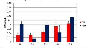
Figure 2.20 Mean ± SE DIN concentrations at all sites before and after channel closure
