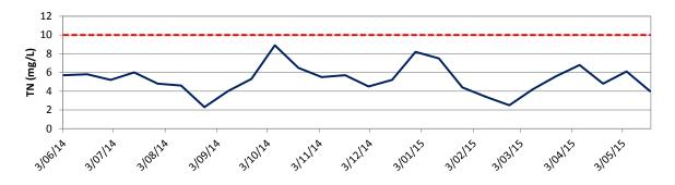
Figure 2.12 Time series of TN concentration from the Evans Head STP discharge (90th percentile limit in red)
