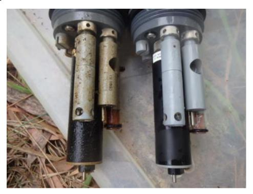
Plate 2.2 Water quality monitoring probes are replaced with a serviced and calibrated spare at two month intervals
