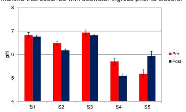
Figure 2.15 Mean ± SE pH at all sites before and after channel closure
