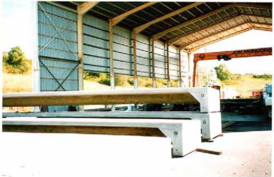
Concept of prefabricated bridges using Doolan Deck modular units
